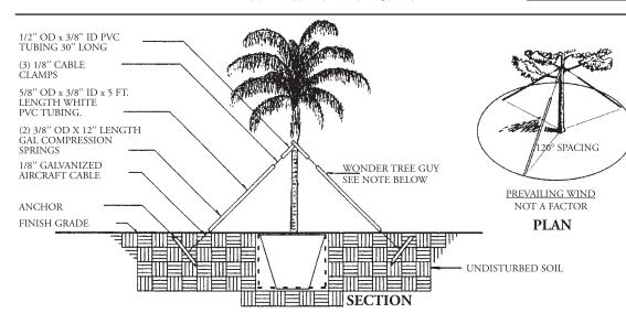
Each Wonder Tree Guy contains (3) 1/8" cable clamps, a Wonder Tree Tie Collar attached to 1/8" 17x19 galvanized steel aircraft cable attached to the 5/8" OD x 5 foot long white PVC tubing attached to the underground anchor. One package contains 3 Wonder Tree Guys.
