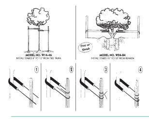
**DESCRIPTION:** MODEL 1446 / 2484; 14/24 COLLAR LENGTH 46'/84' OVERALL LENGTH COMPRESSION SPRING LOADED TREE TIE THAT WILL INSURE THE SAFE AND SUCCESSFUL DEVELOPMENT OF THE NEWLY TRANSPLANTED TREE.
